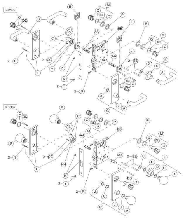
NOTE: L9457, LV9457, and L9466 lock functions have a latch and deadbolt. Lock case and armor front shown with latch and auxiliary latch. L9462 x XL11-886 lock function has deadbolt only. Lock case and armor front shown with latch & auxiliary latch. Standard full face mortise cylinder shown.
