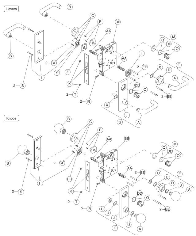
NOTES: L9460 x XL11-886 lock function has a deadbolt only. Lock case and armor front shown with latch, auxiliary latch, and deadbolt. Standard full face mortise cylinder shown.
