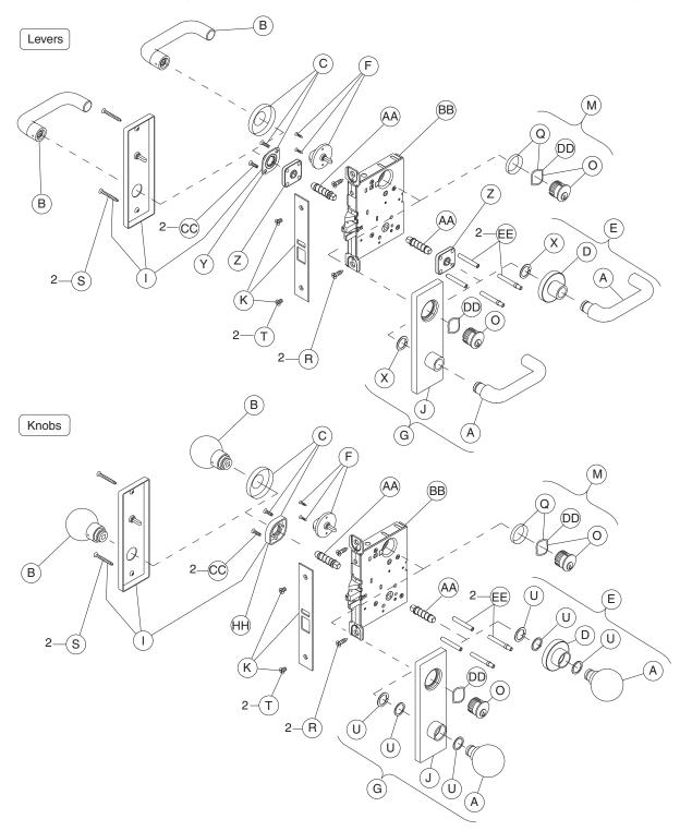
NOTE: L9456, LV9456, and L9473 lock functions have a latch and deadbolt. Lock case and armor front shown with latch and auxiliary latch. L9453, LV9453 lock functions have a latch, auxiliary latch, and deadbolt. Lock case and armor front shown with latch and auxiliary latch only. Standard full face mortise cylinder shown.
