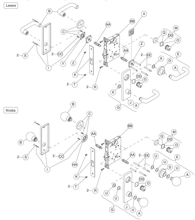
NOTE: L9465 lock function has a latch and deadbolt. Lock case and armor front shown with latch and auxiliary latch.
