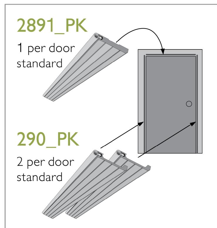
When ordering a head section such as 2891\_PK, two corresponding side sections (290\_PK) should also be ordered for the latch and hinge sides of the frame.
