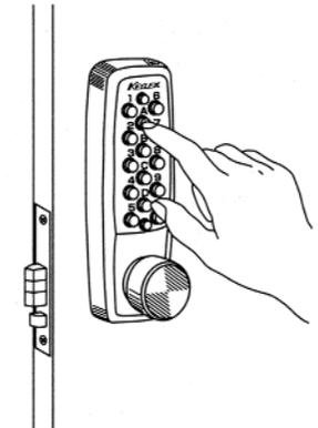
9 Replace the lock body on the door and test all aspects of the locks operation including the new code. Ensure that the door is kept ajar until you are satisfied that the new code operates correctly.
