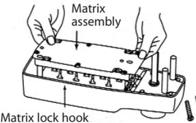
4 Carefully lift the matrix assembly away from the lock body as shown.
