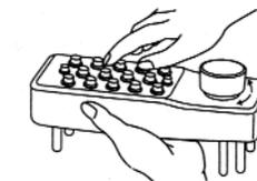
8 Ensure all buttons work smoothly. If any button sticks, check that the code hook has been inserted correctly into its corresponding slot.
