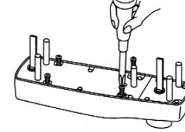
3 Ensure the lock body is horizontal (on its back) and remove the four silver pozi head screws. Re-engage one of these screws into the vacant hole adjacent to the central mounting pillar – this will aid removal of the back plate. **Do not remove any of the Red-cap screws.**
