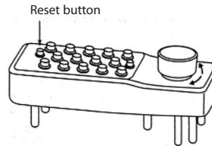
2 Place the lock face down on a bench as shown. Press the Reset button
