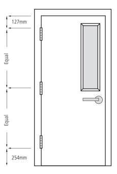
Where door height dictates that additional hinges are required they should be fixed adjacent to and immediately below the top hinge.
