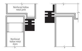
A typical surface mounted installation is shown above (left) where the jamb bracket is fastened to the stop.
