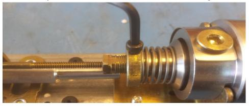
Undo the cap head locking nut and undo the retainer nut as below
