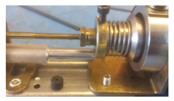
This photo shows the normal position of the plunger and dogging rod, with the latch released. If you now push the push bar you will see the plunger retract. The aluminium rod should have minimum clearance here and act on the latch positively through the dogging rod and when the push bar is fully depressed the plunger should be as below and the latch fully retracted:
