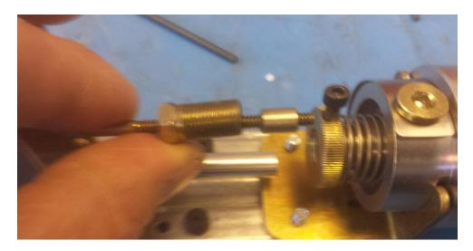
The smooth threaded end stop is the determining factor and should be threaded on with 7 threads showing(as a start point) to the right, before threading the retainer nut back into the knurled nut, you may wish to use threadlock here once set.
