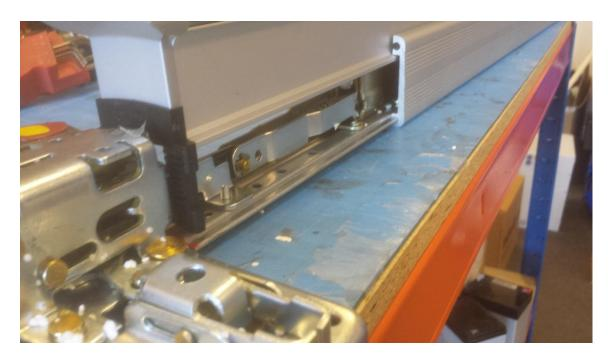
Once the back-plate is free from the housing, lift both plastic guides and support them while holding the push bar and remove it. A sideward and upward movement is required here as the locators have cut-outs to the side.
