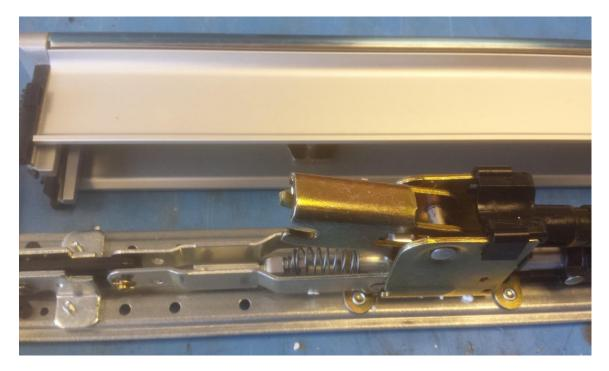
Reinstallation is a reverse of this taking care to lift the plastic guides and not damage them while you slide the back-plate into the aluminium extruded housing.
