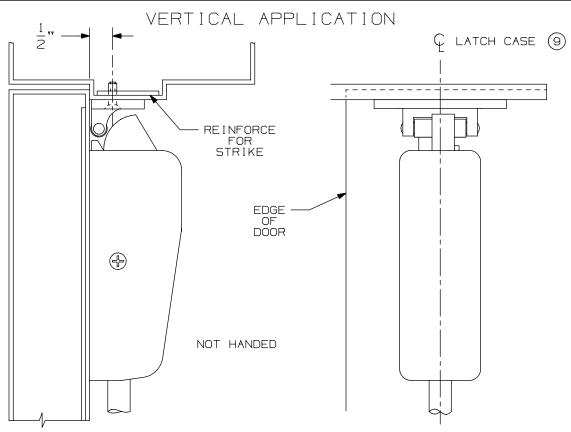
NOTE: LATCH CASE MOUNTING HOLES TO BE PREPARED AT INSTALLATION ON DOOR.
